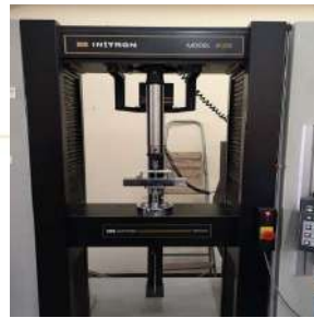
Testing of mechanical strength on bending
