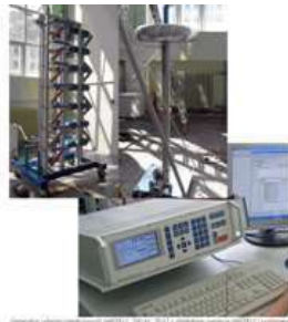
High-voltage tests insulators - shocks
