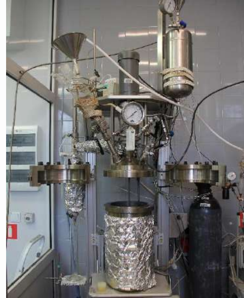
A pressure reactor with a capacity of 15 liters
